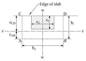
Critical shear perimeter for exterior column
