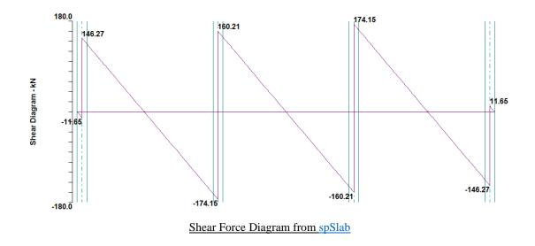
From the shear force diagram, the factored shear force,  $V_{f,c}$ , that is resisted by the exterior and interior columns at a slab-column joint are:
