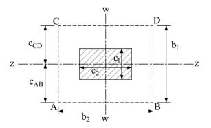
Critical shear perimeter for interior column
